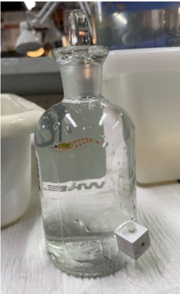
Figure 4. A juvenile krill E. superba in incubation bottle for a respiration/ excretion experiment at Process Study 4. Note port at bottom for oxygen sensor. Photo by Debbie Steinberg.
